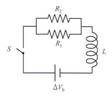
a) The time constant of a series LR-circuit is given by  $\tau = L/R$ . Determine  $\tau$  and its uncertainty for the circuit given above. (7 marks)
