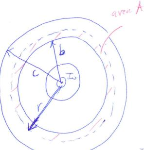
$\oint \vec{B} \cdot d\vec{s} = \vec{B} \lambda \pi r \ exactly \ as$ (1) in (a). Ithrough = Io - JA  $\bigcirc$  $= I_0 - I_0 \pi (r^2 - b^2)$  $\pi(c^2-b^2)$
