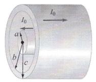
a) Find an expression for the magnitude of magnetic field in the hollow section (a < r < b) of the coaxial cable, where r is the distance measured from the central axis of the cable. Show your work, simply writing down the correct answer will not result in full marks. (4 marks)
