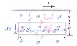
a) Find the magnetic flux through the loop in terms of I and the dimensions given in the figure. (4 marks)
